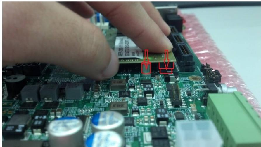
4. After insert the module to the desire slot, drive screws tighten with memory module's crew hole and bolt on PCB board.
